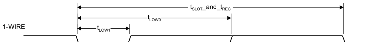
Figure 5-118. 1-Wire Write Bit Timing (Command/Address or Data)
